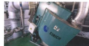
⑥ 造粒器(傾斜回転型ミキサー) Granulator (inclined rotating mixer) 粉塵抑制のため炭化物をφ約 1~3mm に成型します。 The carbide is molded into cylinders about 1~3 mm in diameter to suppress the generation of dust.
